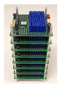
ADLREL-8x16 can be stacked up to eight board high for a total of 8x128 (1024) relays per stack. The ADLREL-CTRL1 mPCle controller can control up to 8 stacks for a total of 8x1024 (8,192) relays.
