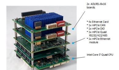
The ADLREL-8x16 PC/104 form factor makes it possible to create compact, rugged complete solutions including Intel Atom and Intel Core CPUs, one or more ADLREL-8x16 boards, and a vast array of PC/104 and mPCle peripheral functionality including:
