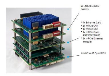
The ADLREL-8x16 PC/104 form factor makes it possible to create compact, rugged complete solutions including Intel Atom and Intel Core CPUs, one or more ADLREL-8x16 boards, and a vast array of PC/104 and mPCIe peripheral functionality including:
