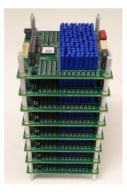
ADLREL-8x16 can be stacked up to eight board high for a total of 8x128 (1024) relays per stack. The ADLREL-CTRL1 mPCIe controller can control up to 8 stacks for a total of 8x1024 (8,192) relays.
