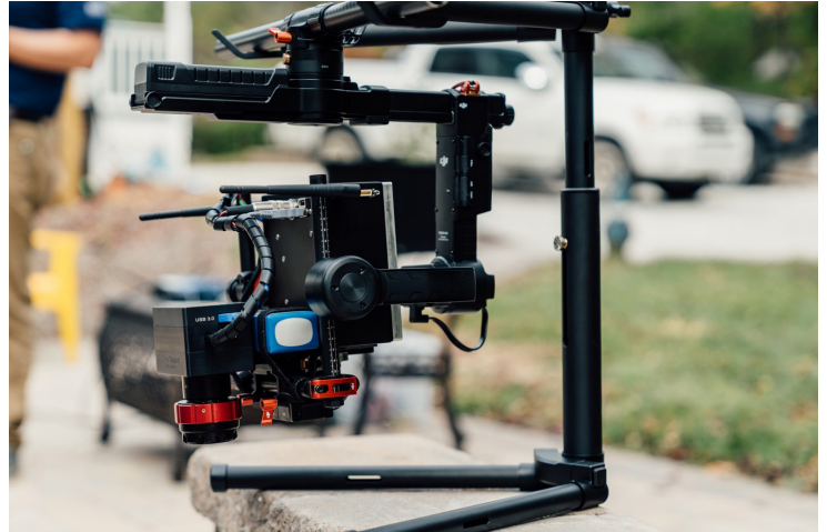
Figure 4: ADL Payload computer with SWIR camera and DJI Ronin MX Gimbal assembly. Drone model used is DJI Matrice 600. 4,5
